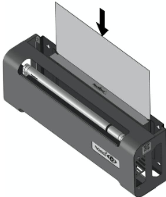
4. Make sure that the folded section bends down to a right angle at the bottom of the channels, and the top edge of the sticky board is level with the top edge of the metalwork, and not protruding beyond it.
