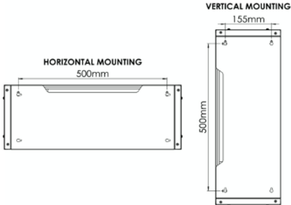
Mark off the necessary fixing points onto the mounting surface using the paper mounting template provided. Drill holes to a depth of 40mm using a 5.5mm drill bit. Place the plastic plugs into the wall, then screw the screws into the plugs leaving the head of the screw approximately 10mm from the wall. The trap will now hook over the screws using the keyhole feature.
