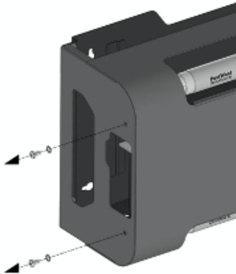
3. Align the ceiling suspension bracket with the screw holes and reinsert the screws and washers using a pozi-drive screwdriver. Ensure the screws are tightened securely.
